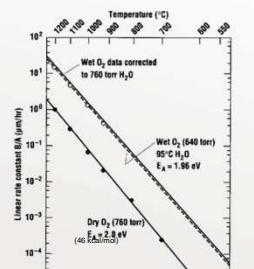
Figure 4.3 Arrhenius plot of the ratio (B/A) of the oxidation parameters (after Deal and Grove). (111) wafers
