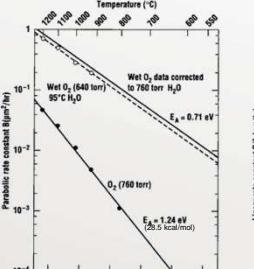
Figure 4.2 Arrhenius plot of the B oxidation coefficient versus  $1000/T (\text{K}^{-1})$ . The wet parameters depend on the  $\text{H}_2\text{O}$  concentration and therefore on the gas flows and pyrolysis conditions (after Deal and Grove). (111) wafers
