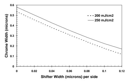
Figure 1: Design curves for a rim shifted 0.5  $\mu$ m isolated line for the two listed exposure doses (i-line, NA = 0.5,  $\sigma$  = 0.4, SPR500 resist, bare Si wafer, simulated with PROLITH/2).
