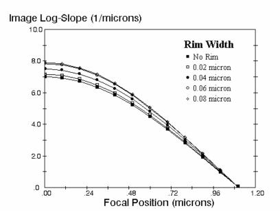
Figure 4. Log-slope defocus curves for a 0.35  $\mu$ m line/space array for varying amounts of rim shifter width (i-line, NA = 0.5,  $\sigma$  = 0.4, using chrome width as determined from the design curves of Figure 2, simulated with PROLITH/2).
