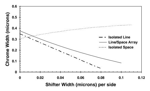
Figure 2: Design curves for rim shifted 0.35  $\mu$ m features (i-line, NA = 0.5,  $\sigma$  = 0.4, SPR500 resist, bare Si wafer, 200 mJ/cm<sup>2</sup> exposure dose, simulated with PROLITH/2).
