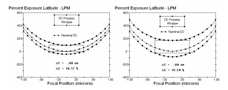
Figure 6. Comparison of process windows generated using the Lumped Parameter Model (LPM) for (a) no rim, and (b) a 0.1  $\mu$ m rim for a nominal 0.4  $\mu$ m isolated space (i-line, NA = 0.5,  $\sigma$  = 0.4, simulated with PROLITH/2)
