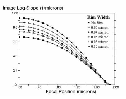
Figure 5. Log-slope defocus curves for a 0.35  $\mu$ m isolated space for varying amounts of rim shifter width (i-line, NA = 0.5,  $\sigma$  = 0.4, using unshifted space widths as determined from the design curves of Figure 2, simulated with PROLITH/2).
