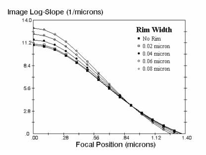
Figure 3. Log-slope defocus curves for a 0.35  $\mu$ m isolated line for varying amounts of rim shifter width (i-line, NA = 0.5,  $\sigma$  = 0.4, using chrome width as determined from the design curves of Figure 2, simulated with PROLITH/2).
