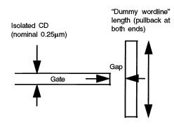
Figure 2. Test pattern containing features for measuring pullback. Nominal CD is  $0.25\mu$ m. Drawn features are polysilicon : on the mask, they are opaque on a clear background
