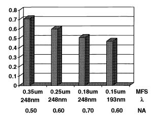
Figure 1. Decrease in  $k_1$  factor (from the Rayleigh relation) with process generation. A smaller  $k_1$  indicates more challenging lithography, i.e., the need for greater resolution relative to the basic capability of the optical system.
