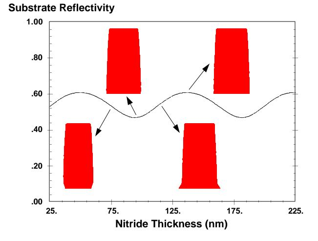
Figure 3. Nitride thickness also affects the shape of the resist profile, causing resist footing, undercuts, or vertical profiles. Substrate reflectivity (the square of the magnitude of the reflection coefficient) is shown for comparison.
