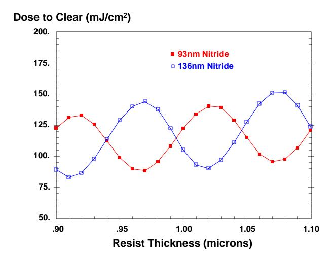
Figure 2. Changes in nitride thickness cause a shift in the phase of the resist swing curve, making nitride thickness control as critical as resist thickness control.
