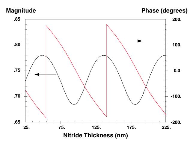
Figure 1. Variation of the magnitude and phase of the resist/substrate reflection coefficient as a function of silicon nitride thickness for a film stack of resist on nitride on 40nm of oxide on silicon.
