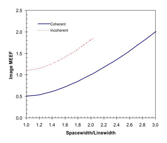
Figure 2. The impact of duty cycle (represented here as the ratio of spacewidth to linewidth for an array of line/space patterns) on the image CD based MEEF for both coherent and incoherent illumination. For the incoherent case, an  $MTF_1$  of 0.45 was used.
