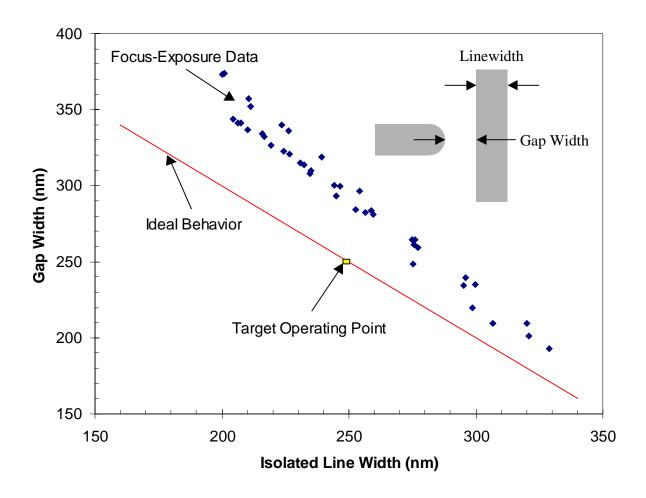
Figure 2. Line end shortening can be characterized by plotting the gap width of a structure like that in the insert as a function of the isolated linewidth under a variety of conditions. As shown here, changes in focus and exposure produce a linear gap width versus linewidth behavior.
