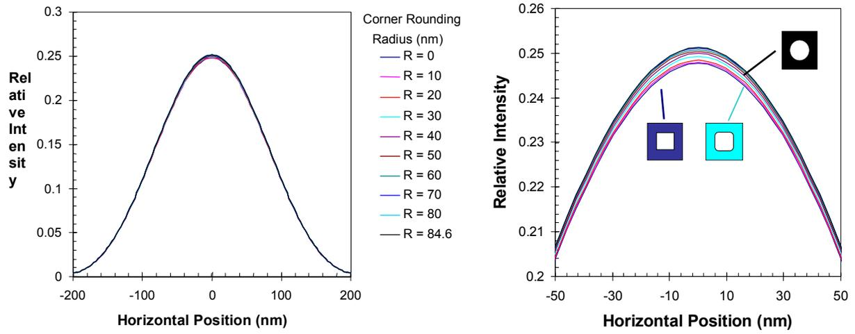
Figure 1. Aerial image results as a function of corner rounding radius ( $\lambda = 248\text{nm}$ ,  $\text{NA} = 0.7$ ,  $\sigma = 0.4$ , isolated  $150\text{nm}$  contacts) shown at two different graph scales. For all masks, the area of the contact hole remained constant.
