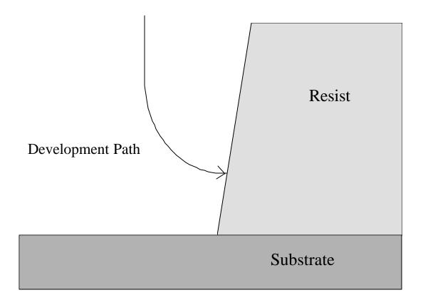
Figure 1. Typical development path starts out vertically, but ends up nearly horizontal by the end of the development cycle.
