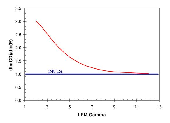
Figure 2. A plot of equation (4) showing how the exposure latitude term approaches its limiting value of 2/NILS as the lumped photoresist contrast increases. In this case, the resist aspect ratio is 2, the ratio I(CD/2)/I(0) is 0.5 and the NILS is 2.
